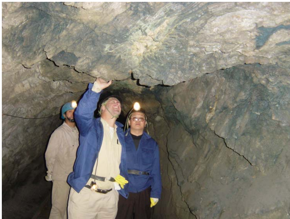
Figure 2: Inspecting massive sulphide copper mineralisation 240 metres below surface at the small Cai Hua Gou mine (excised from the centre of the Copper Mountain project area).
